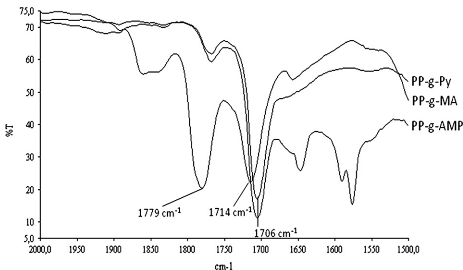
Fig. 2. FTIR spectra of PP-g-MA, the product of the reaction between PP-g-MA and the amino-pyrene derivative (PP-g-Py) and the product of the reaction between PP-g-MA and aminomethylpyridine (PP-g-AMP).
